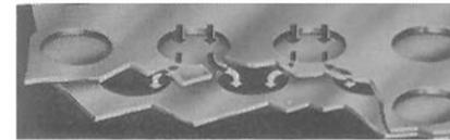
**Neva-Clog®** is a unique metallic filter medium consisting of two perforated sheets with offset holes. The smooth surface resists abrasion and promotes easy cake drop. Neva-Clog does not easily blind, clog or corrode. It is usually made of 316L.
